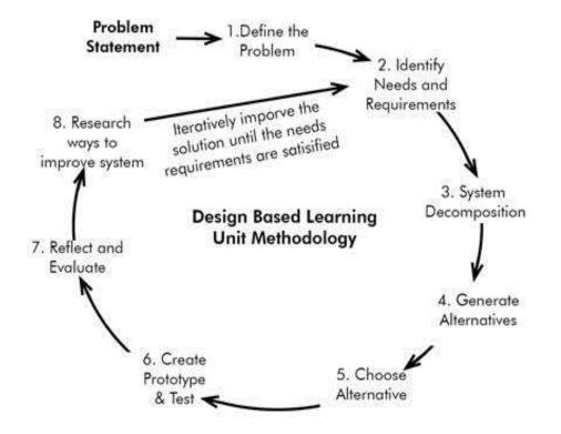
The DBL provides a working, tested framework upon which Robot Algebra design problems are built. They provide a natural mode for teaching the topics which are inherent to robotics and technology and have proven success in the classroom over several years of research and refinement.
